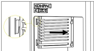
① Insert the grill rack, aligning the buckles on its rear end with the slots on the inner wall of the appliance.
