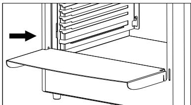
① Align the buckles on the side of the work table with the slots on the appliance.
