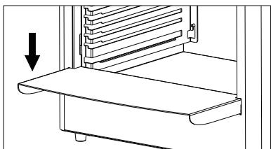
② Gently lower the work table into place to complete installation.
