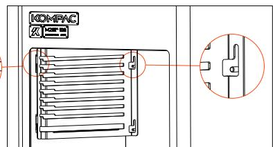
② Insert the front buckles of the grill rack bracket into the slots on the inner wall.
